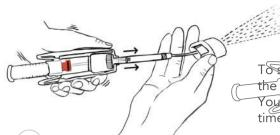
To spray: Fully compress and hold the levers.
